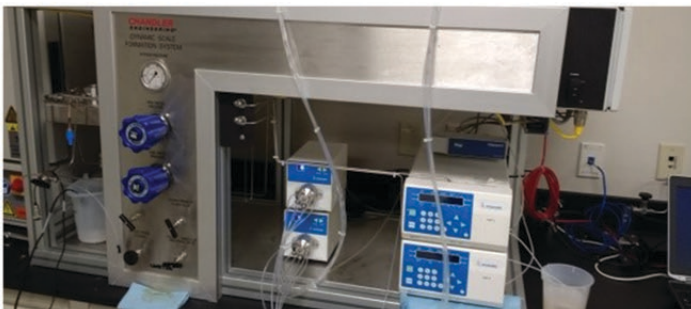
Dynamic scale loop: Scale Inhibition: Dynamic scale loop to determine effectiveness of inhibitors and compatibility of comingling waters
