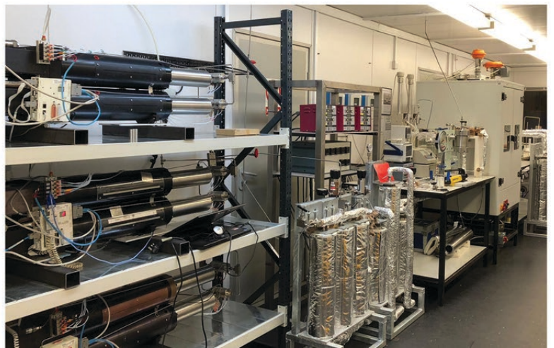
Dynamic scale loop: Scale Inhibition: Dynamic scale loop to determine effectiveness of inhibitors and compatibility of comingling waters
