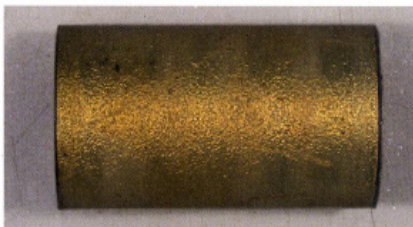
24-carat gold film prevents gas leaking from the core under hydrothermal conditions
